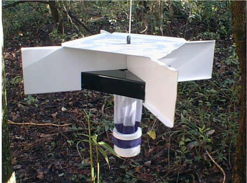
Figure 1. Omni-directional Fay Prince trap with collection cup.
