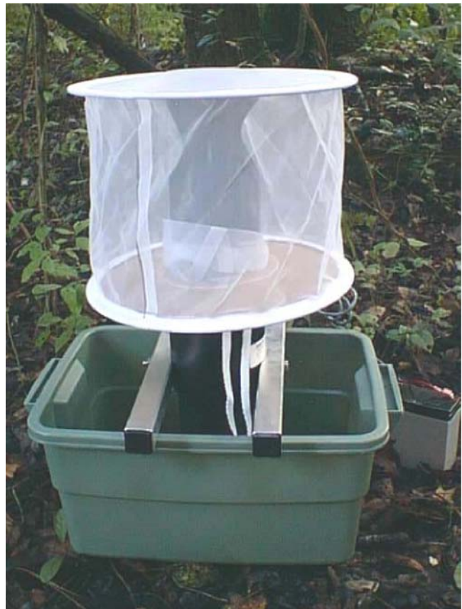
Figure 1. The CDC Gravid Trap with a 6 Volt, 10 AmpHr battery.
