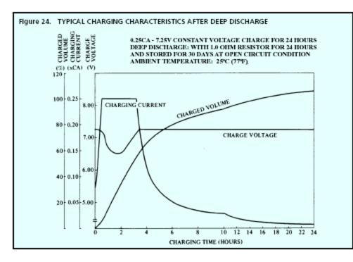
When a battery has been subjected to deep discharge (commonly referred to as overdischarge), the amount of electricity which has discharged been is actually 1.5 to 2.0 times as great as the rated capacity of the battery. Consequently, a battery which has been overdischarged requires a longer charging period than normal. Please note, as shown in Figure 24 below, that as a result of internal resistance. charging current accepted by an over-
