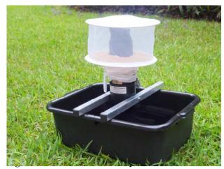
rim of the pan with the shorter tube without the large holes in the sides protruding downward (see figure). Next, slip the collection bag over the upright tube and slide the sleeve downwards towards the aluminum supports until the "bottom" of the bag is resting on the top end of the trap as shown. The final step, after adding the oviposition medium described below, is to connect the trap to a 6 volt DC source, being careful to observe correct polarity (see below).
