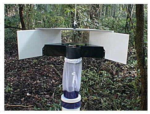
wind-orienting cover and cylinder housing a suction motor and suspending the collection bag.
