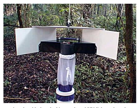
design is based on the attraction of contrasting gloss black and white panels and UV light, and employs a wind-orienting cover and cylinder housing a suction motor and suspending a collection bag or killing jar.
