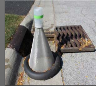
Figure 3: Image of large emergence trap used in roadside catch basins before being placed on water.
