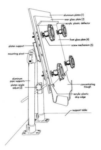
The figure to the left shows the vertical aluminum pipe support with the slotted arm attached to the back of the platen (1).
