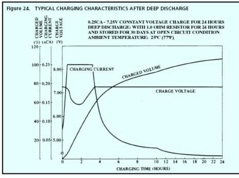
When a battery has been subjected to deep discharge (commonly referred to as overdischarge), the amount of electricity which has been discharged is actually 1.5 to 2.0 times as great as the rated capacity of the
