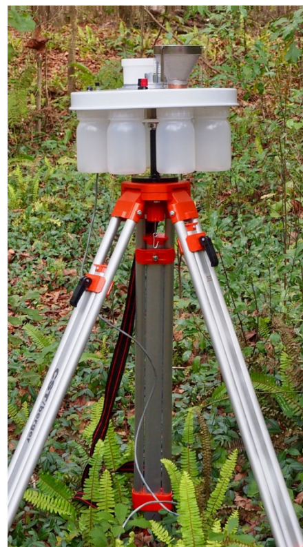
Figure 1. Collection Bottle Rotator mounted on tripod and machined adapter, P/N 1512.5
