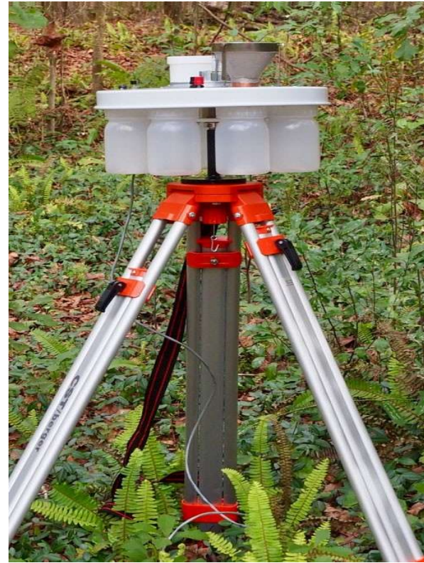
Figure 1. Collection Bottle Rotator , PN 1512 mounted on the Tripod and powder-coated adapter , PN 1512.50.
