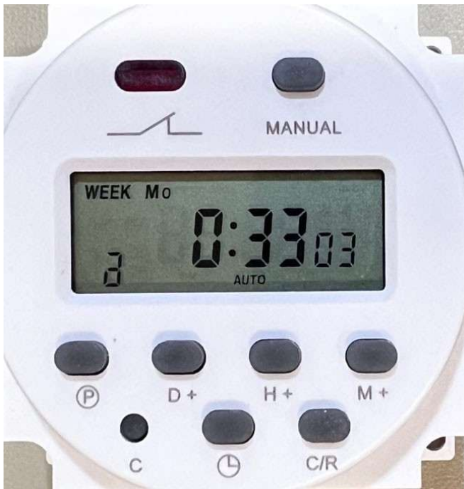
Figure 2. The Digital Programmable Timer Switch of the Collection Bottle Rotator PN 1512 manufactured after 2024. Note, the display of the \partial symbol (lower left in LED screen) indicates that the Timer Switch is in the LOCKED state; pressing the C/R button four (4) times until the \partial symbol disappears will UNLOCK switch permitting the buttons to be used to program the CBR's Timer Switch.
