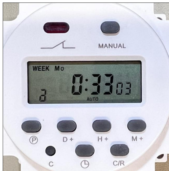
Figure 1. The digital programmable timer switch of the Collection Bottle Rotator.
