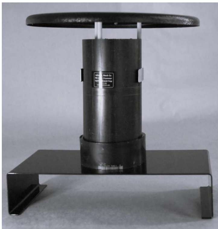
Figure 1. The Improved Frommer Updraft Gravid Trap Model 1719 incorporates all of the features of the original CDC Gravid Trap (our Model 1712) with an important modification—the collection chamber is below the aspiration fan. Not shown here is the black pan for holding the oviposition media (see Fig. 3)
