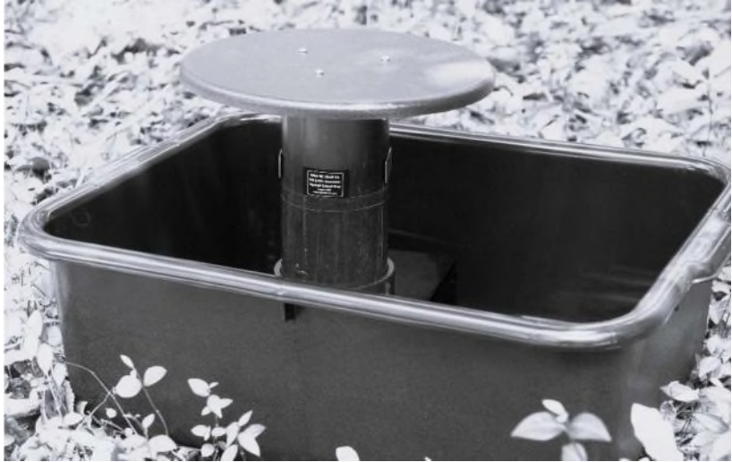
Figure 3. The complete Improved Frommer Gravid Updraft Trap shown in the pan holding the oviposition solution. The required battery is not shown.
