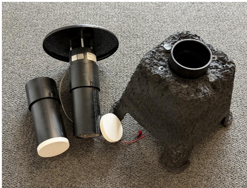
Figure 2. Improved CDC Resting Trap Model 1732 comes complete with aspirator body with rainshield, wood-fiber resting box with couple, and two collection chambers.
